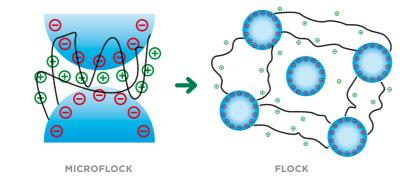
The flocculants are high molecular weight polymers that are capable of trapping various colloidal particles in its polymer chain.
